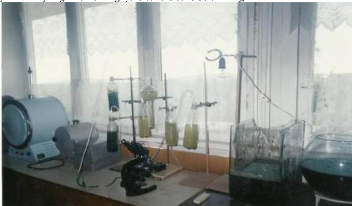
1- rasm Xlorellani laboratoriya sharoitida o'stirish qurilmasi
