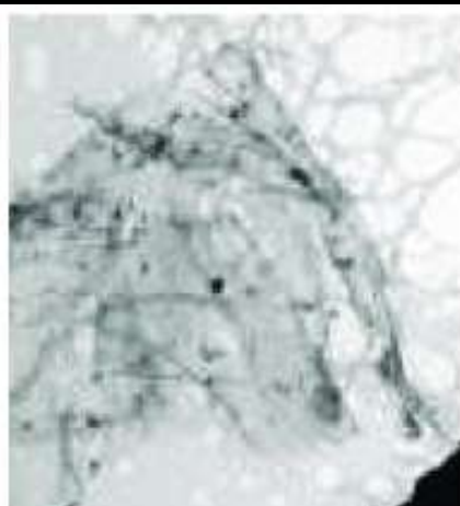
Figure 19. Microscopic image of soot obtained from methane
