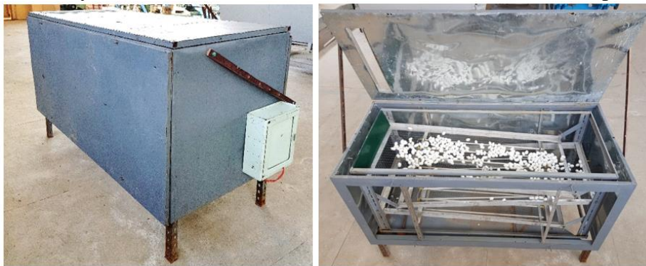
Figure 3. Infrared vibrating drying unit for the primary treatment of mulberry silkworm cocoons
