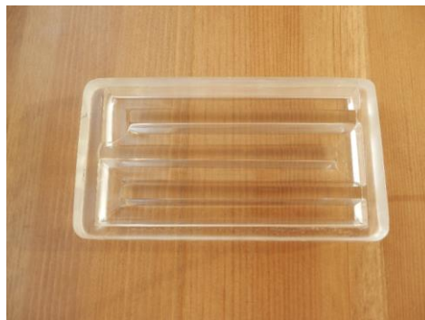
4-rasm. Labirint shaklidagi chuqurchaga ega bo'lgan bogorov kamerasi
