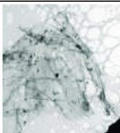
Figure 19. Microscopic image of soot obtained from methane
